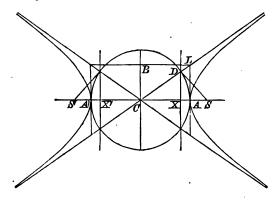
99. Prop. VI. The asymptotes intersect the directrices in the same points as the auxiliary circle, and the lines joining the corresponding foci with the points of intersection are tangents to the circle.
